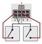
A change-over contact can also be used for running products both up and down but stops are not possible, for instance for a thermostat.
