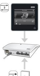
If you **only** have a VELUX INTEGRA® one-way remote control (labelled with the symbol ), you can copy the products operated by this control to the interface. See how on pages 17-19.
